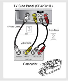
This figure shows the Standard connector-jack panel. The actual configuration for your TV may be different.
